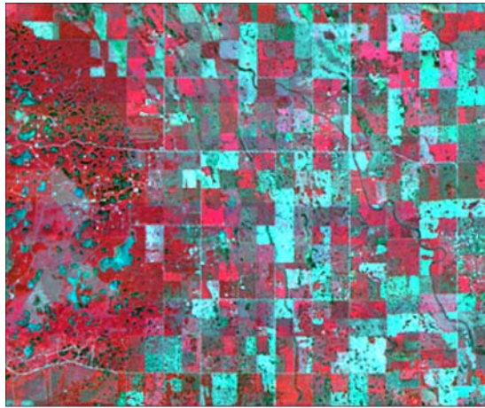
56-Meter Pixel AWIFS Satellite Image Displayed: Band 3-IR, 2-red, 1-green
